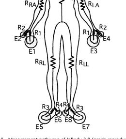
**Figure 1** Measurement pathways of InBody 3.0 (graph reproduced by courtesy of Biospace). The subject stands with her or his soles in contact with the foot electrodes and grabs the hand electrodes.  $R_{RA}$ , resistance of right arm;  $R_{T}$ , resistance of trunk;  $R_{LA}$ , resistance of left arm;  $R_{RL}$ , resistance of left leg. See text for details.
